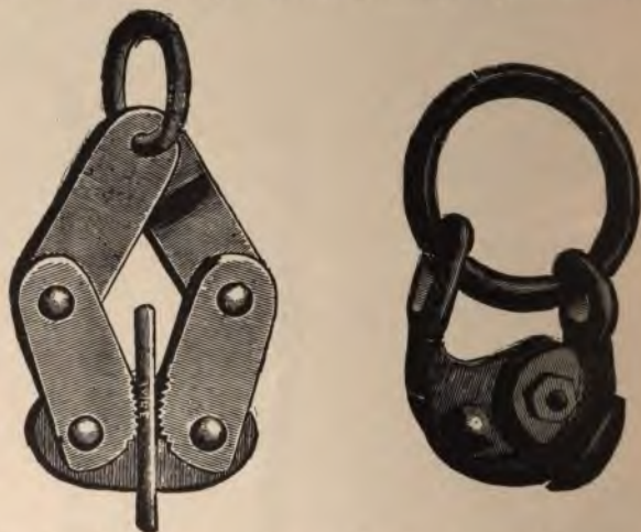
FIGS. 235-236.—Two forms of "come-along." The wire is inserted between jaws and is held fast when tension is applied to the ring.
